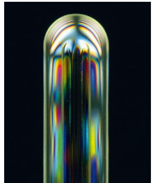
Special tempered MAXOS® glass under polarized light.
